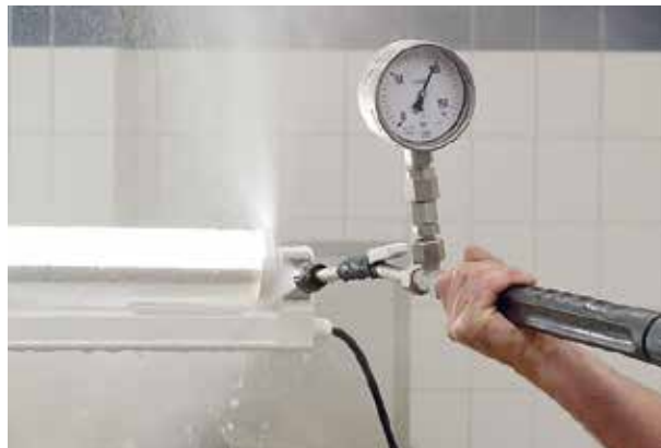
> High-pressure cleaning of housing cover with 100 bar
